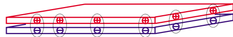
FIG. 1. (Color online) A schematic picture of DEC. An exciton forms as a result of the pairing of an electron in an electron-rich layer and a hole in a hole-rich layer.
